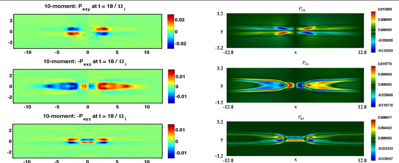
Off-diagonal components of the electron pressure tensor for our 10-moment simulation at  $\Omega_i t = 18$
