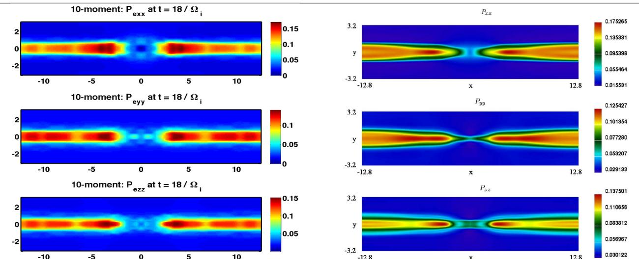
Diagonal components of the electron pressure tensor for our 10-moment simulation at  $\Omega_i t = 18$
