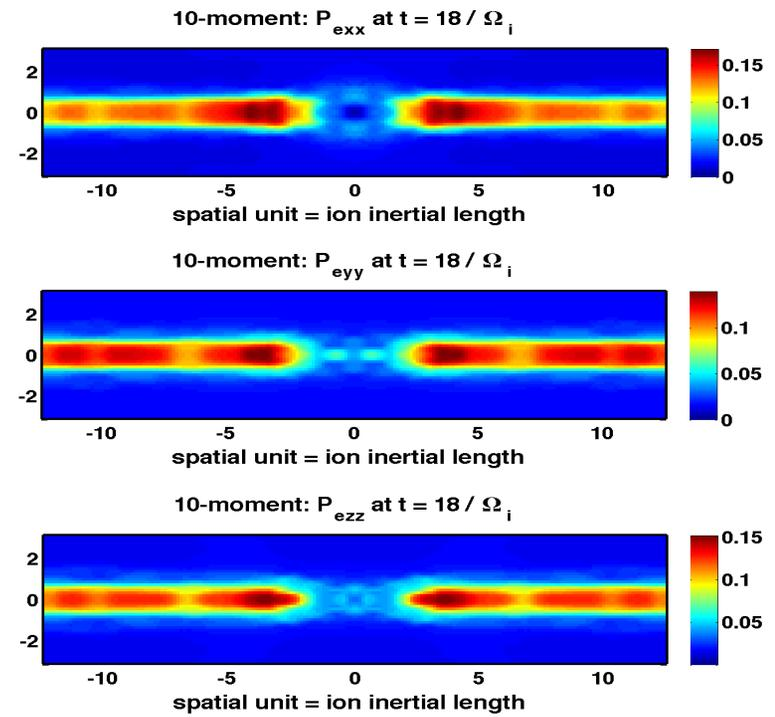
Diagonal components of the electron pressure tensor for 10-moment simulation at  $\Omega_i t = 18$
