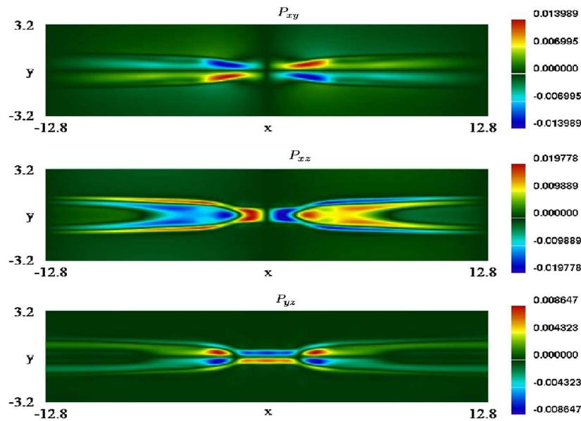
Off-diagonal components of the electron pressure tensor for Vlasov simulation at  $\Omega_i t = 17.7$  [ScGr06]
