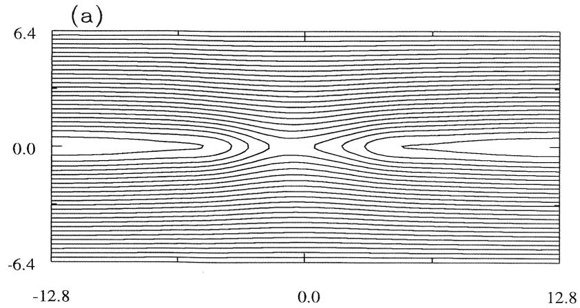
Magnetic field lines for PIC at  $\Omega_i t = 15.7$  [Pritchett01]
