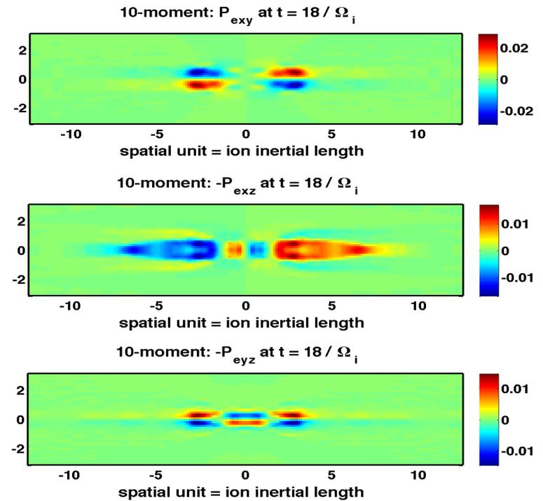
Off-diagonal components of the electron pressure tensor for 10-moment simulation at  $\Omega_i t = 18$
