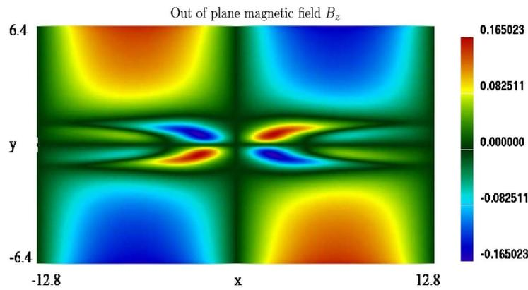
Magnetic field for Vlasov at  $\Omega_i t = 17.7$  [ScGr06]
