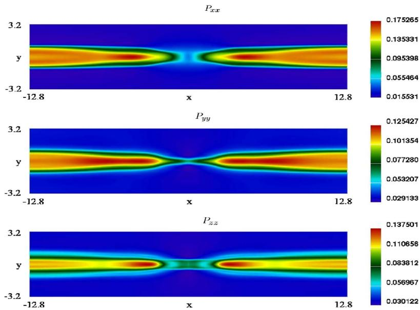
Diagonal components of the electron pressure tensor for Vlasov simulation at  $\Omega_i t = 17.7$  [ScGr06]
