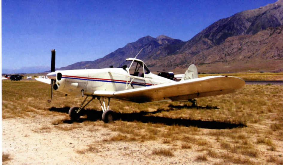
"Worst bent prop I've ever seen." Pawnee damaged by instant violent updraft during the start of a tow at Nephi, Utah. The airport is surrounded by thousands of acres of green farmland - which would not provide any dirt to make a visible "dust devil" out of any strong vertical vortex convection that might be pushed by a cross wind onto the runway. Any surface - bare rock, pavement, green cropland, whatever - can produce invisible vertical vortex convection events that can catch pilots and ground crews off guard. Photo by Bob Thompson
